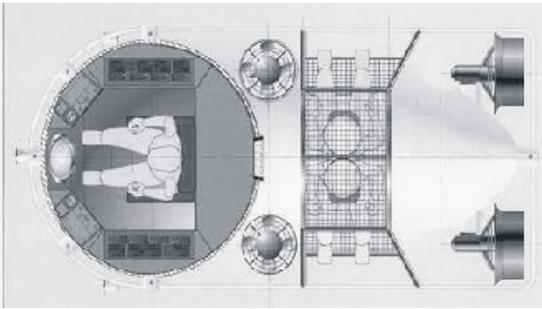
**Graph 12.** A view from top of «Fast Diver». A pilot in a durable compartment with normal pressure. Two divers-rescues in a “wet” compartment (using liquid ventilation devices). They can go up and down fast (together with escaping submariners).
