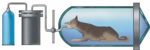
**Graph 6.** Model of portable liquid ventilation device connected to transparent capsule filled with water. 10 experiments were worked out to learn the imitation of compartment flooding while staying under
